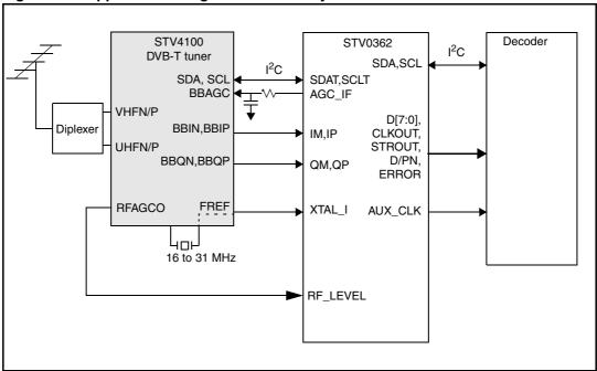
Figure 1. Applications diagram for DVB-T system
