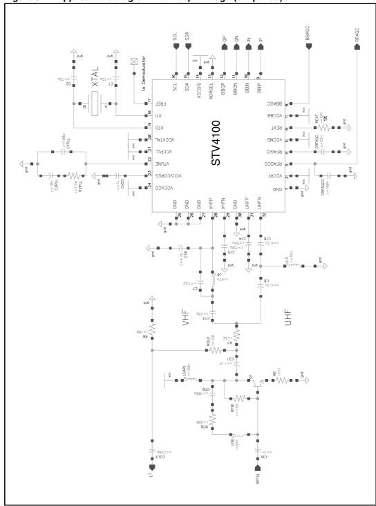
Figure 3. Applications diagram with loop-through (simplified)
